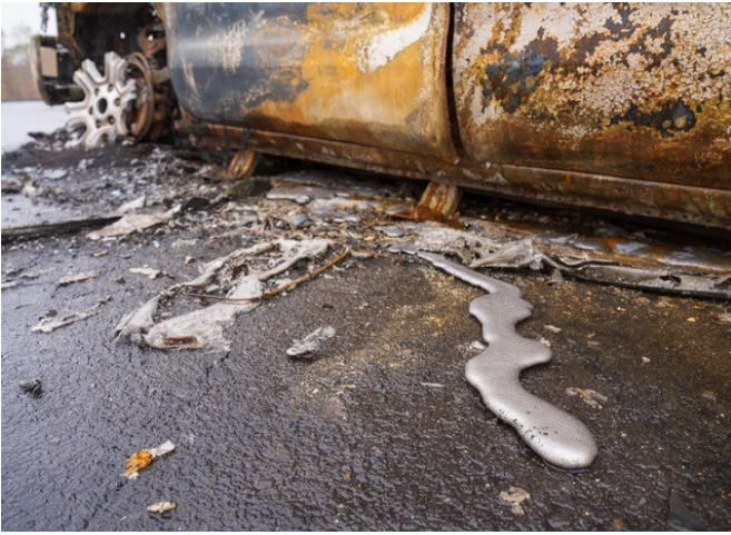
Someone tried driving along Hammonds Plains Road during the fire and their vehicle caught fire. It was hot enough to melt the aluminum.
